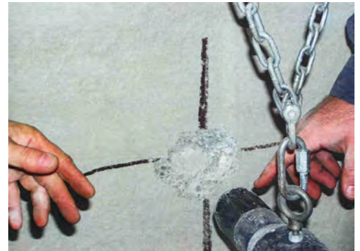
Reinforced precast wall after 150 impacts
